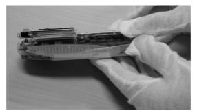
Place the display assembly on top of the PWB inside the D-cover.
