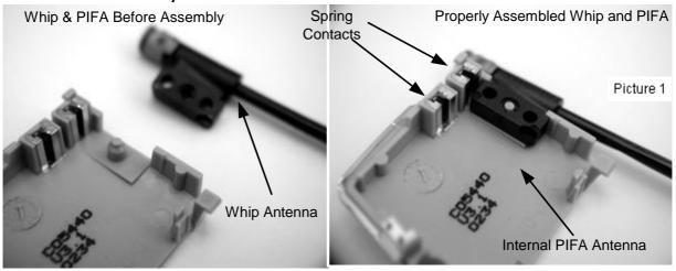
1. Snap whip Antenna onto Internal antenna as shown in Picture 1.
