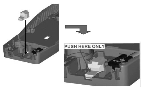
*Caution: The microphone assembly is loose in the D-cover. Don't turn the phone over unless the PWB and display assemblies have been re-installed.*
