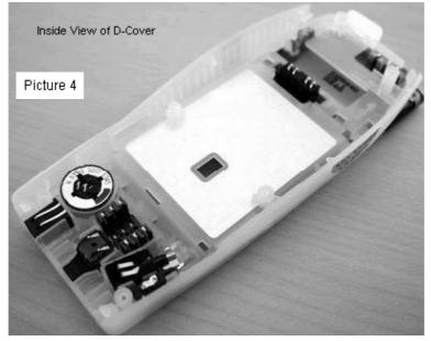
If any of the parts within the D-cover assembly have been removed, insert new parts into their proper locations (as shown in Picture 4). The following diagrams (a through i) illustrate in detail the insertion procedures for each assembly part.
