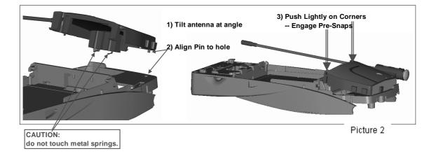
2. Align and insert tip of antenna assembly onto the D-cover as shown in Picture 2. *Make sure antenna spring contacts are not bent or broken.*
