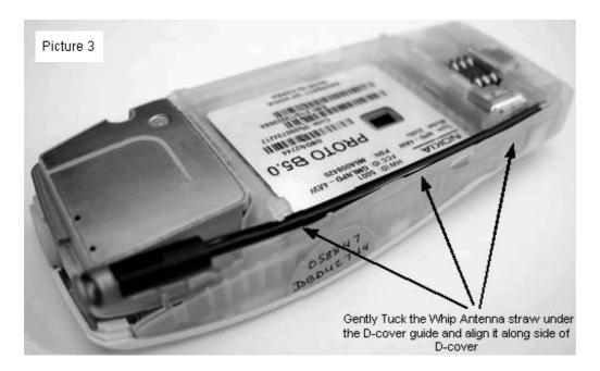
5. Finally, align the whip under the antenna guide and ensure it is remains in place without any additional aid. (See picture 3.)
