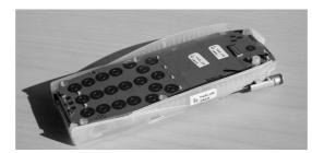
Place the PWB assembly inside the D-cover, making sure it is correctly aligned.
